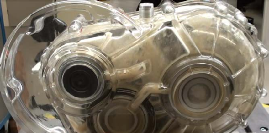
Figure 2: Transmission for lubrication tests with RP plastic gears
