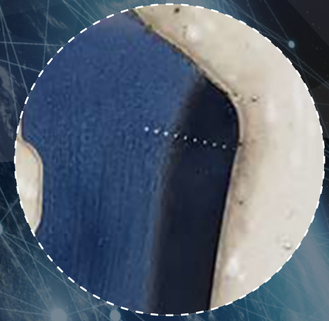
Microscopy of manually manufactured inductor coil shows hardening profile with varying hardness penetration depth
