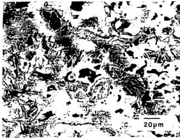
Figure 13 : Partially alloyed material (Distaloy 4800A) + 0.4% graphite, single pressed, sintered at 2050°F. Etched in 2% nital/4% picral.
