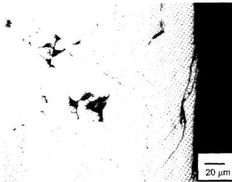
Figure 12: Microstructure of Green Compact near Die-Wall for Material IA-Lubricated Powder with 0.75 w/o Admixed S Lubricant
