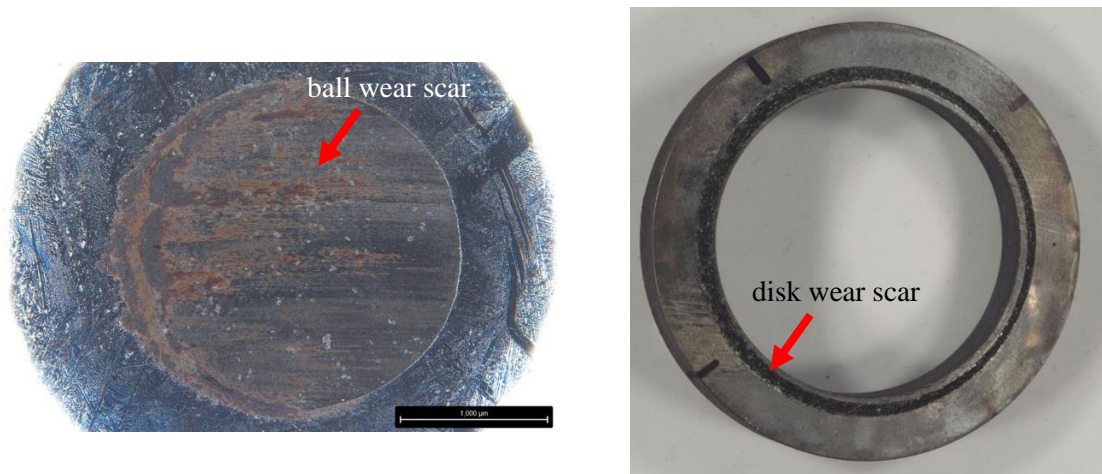
Figure 13. Images of AISI 52100 ball (left) and disk (right) after testing.
