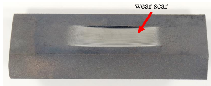
Figure 11. Image of abrasion sample after testing.
